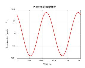
**3** The figure shows readings from accelerometers attached to the base and platform of a vibration isolation table.
