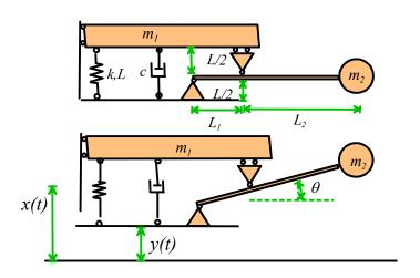
4.1 Draw free body diagrams showing the forces acting on the mass  $m_1$  and the pendulum assembly (see the figure).
