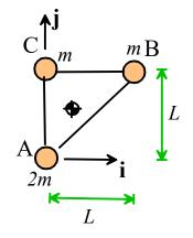
7.1 Calculate the position of the center of mass of the assembly
