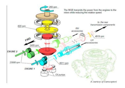
**5.** <u>This paper</u> (VPN connection to Brown required) describes a planetary gear system in a helicopter (see the figure). The ring gear in both epicyclic gears are stationary. The figure shows the angular speeds of the sun and planet carrier on the two systems. Select numbers of teeth for the ring, sun and planet gears in the two epicyclics (find the lowest possible numbers of teeth on each gear).
