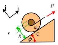
3.1 Draw a free body diagram showing the forces acting on the spool
