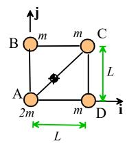
8.1 Calculate the position of the center of mass of the assembly
