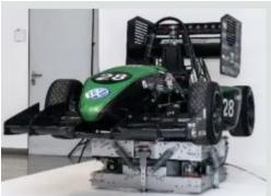
**5.** The figure shows a simplified idealization of a <u>commercial instrument</u> for measuring the inertial properties of large objects. It operates by measuring the amplitude and frequency of small oscillations of a platform, together with the horizontal and vertical reaction forces at the pivot.
