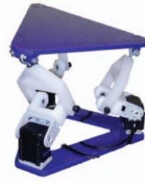
(b) Motion simulation platform (the joints connecting the platform to the members beneath it are spherical joints. The rest are all pin joints)
