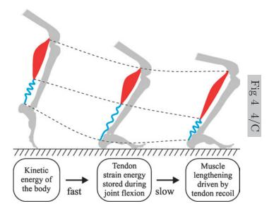
**Figure 4.** Schematic summary of the tendon buffering mechanism. Energy is absorbed initially by the tendon during a brief and rapid event, followed by a relatively slow flow of energy from the tendon to the muscle as fascicle lengthens and dissipates energy.
