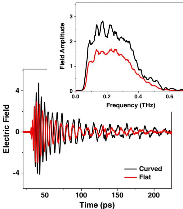
**Fig. 2** Typical time-domain THz signals at the output of a flat-surface and curved-surface ( $R = 6.7$  cm) waveguide measured on axis. The corresponding amplitude spectra are shown in the inset.
