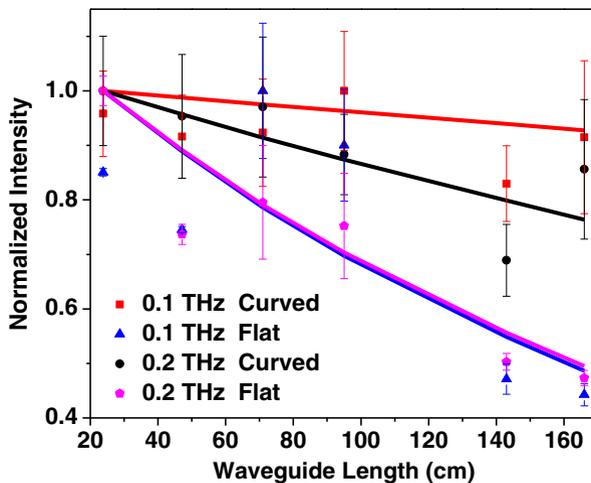
**Fig. 5** Normalized integrated intensity at 0.1 THz and 0.2 THz, at specific points along the length of the flat-surface and curved-surface waveguides. The solid curves are exponential fits.
