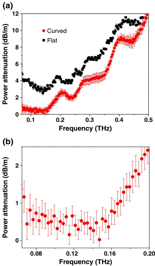
**Fig. 6** (a) Estimated power attenuation for the curved-surface (red circles) and flat-surface (black squares) waveguides. (b) Zoomed in view of the range between 0.07 THz to 0.20 THz for the curved-surface waveguide.
