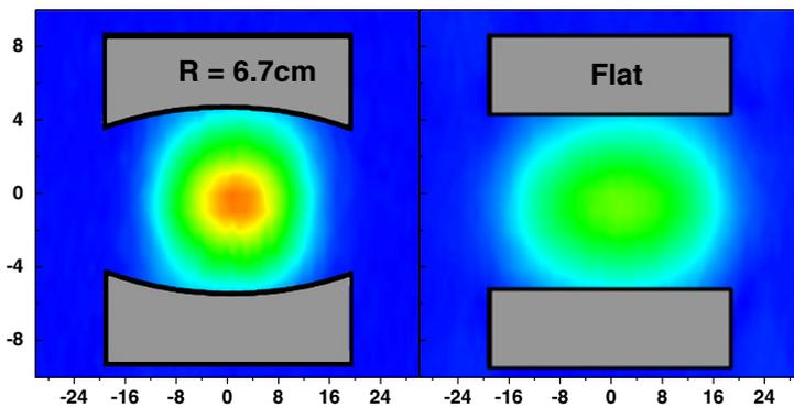
**Fig. 3** Two dimensional color plots showing the electric field distribution at a frequency of 0.1 THz, measured across the output facet of (a) a 24 cm long curved-surface and flat-surface waveguide, and (b) a 167 cm long curved-surface and flat-surface waveguide. The grid dimensions are given in mm.
