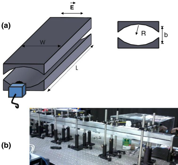
**Fig. 1** (a) Schematic of the curved-surface waveguide where the input electric field is polarized parallel to the inner plate surfaces to excite the TE<sub>1</sub> mode. The THz receiver is shown scanning across the output facet. The inset shows the cross-sectional view of the waveguide. Note that the degree of curvature is exaggerated for clarity. (b) Photograph of the fully assembled curved-surface waveguide.
