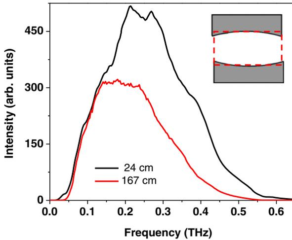
**Fig. 4** Integrated intensity spectra of the measured waveforms at the output of the curved-surface waveguide, within a  $10 \times 40$  mm grid as shown in the inset. The black and red curves correspond to a length of 24 cm and 167 cm, respectively.
