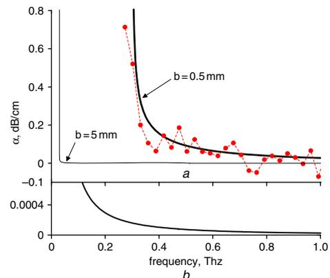
**Fig. 2** Attenuation constant for TE<sub>1</sub> mode, and baseline of theoretical curve
