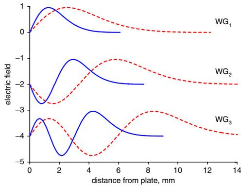
**Fig. 7** Spatial electric field profiles of three lowest-order TE-type WG modes at 0.1 THz (dashed curves) and 0.3 THz (solid curves) based on theory (profiles vertically offset for clarity)
