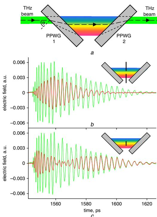
**Fig. 10** Device geometry showing two complementary PPWGs; typical time-domain output signal and reference in bandpass configuration, and in band-stop configuration
