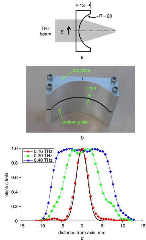
**Fig. 9** Schematic of PPWG-lens; photograph of fabricated device; derived experimental electric field profiles
