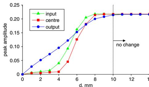
**Fig. 6** Peak positive amplitude of propagated signal as a function of slit opening  $d$ , formed at input, centre, and output of curved plate (no change in signal after 10 mm)
