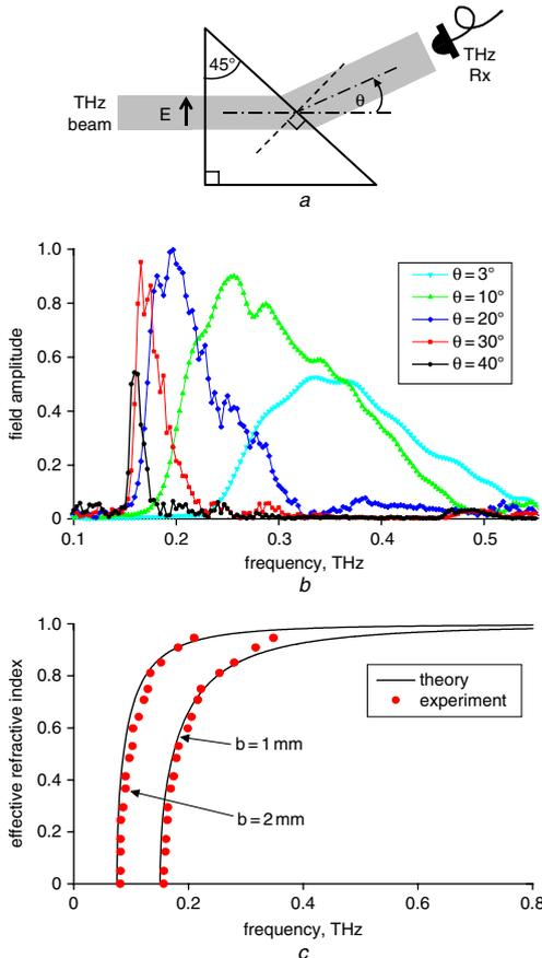
**Fig. 8** Schematic of PPWG prism; amplitude spectra; effective refractive index
