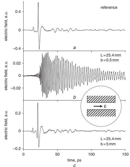
**Fig. 1** Time scans corresponding to (Fig. 1a) input reference, and TE<sub>1</sub>-mode propagation in 25.4 mm long PPWG with (Fig. 1b)  $b = 0.5$  mm, and (Fig. 1c)  $b = 5$  mm
