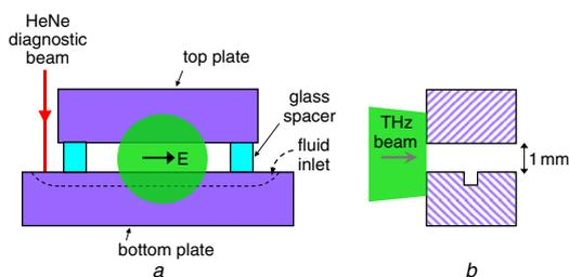
**Fig. 3** Input face of assembled PPWG, and axial cross-section of device
