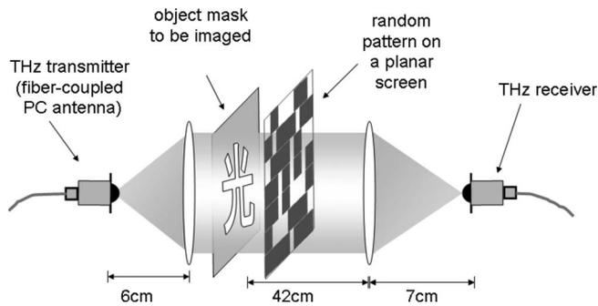
FIG. 1. The terahertz compressive imaging setup. An approximately collimated beam from the terahertz transmitter illuminates an object mask and is partially ( $\sim 50\%$ ) transmitted through a random pattern of opaque pixels. The random patterns, the focusing lens and the receiver, are placed in order to most efficiently focus the terahertz beam onto the receiver antenna. We collect one complete time-domain waveform for each random pattern.
