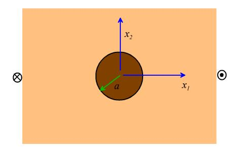
An infinite solid contains a rigid cylindrical inclusion of radius *a* at the origin. The solid is subjected to remote anti-plane shear loading:
