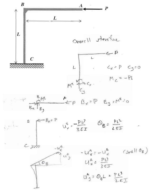
4. A roller support is added at point A. Determine the reactions at point A and C.
