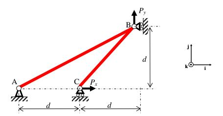
c. Find the potential energy for the structure as a function of the nonzero displacement components of joints B and C, and any of the other parameters of the problem.
