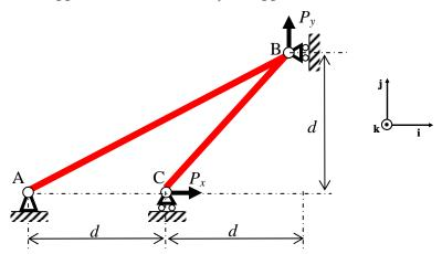
a. Is this truss statically determinate, indeterminate, or a mechanism? Why?
