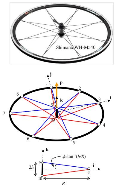
A load *P* is applied to the hub (node 9) in the **k**-direction. As a result, nodes 9 and 10 undergo corresponding displacements  $(u_1^9, u_2^9, u_3^9) = (u_1^{10}, u_2^{10}, u_3^{10}) = (0, 0, u_z), \quad u_z \ll L_0.$
