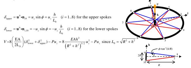
b. Find the hub displacement  $u_Z$  as a function of P, E, A, h, and R. (2 points)
