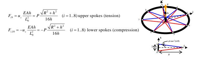
d. Suppose you want to take into account the hub elasticity. The hub is made from the same material (Young's modulus *E*) and has cross sectional area of  $A_h=16A$ . Write the potential energy of the wheel (spokes, hub, and load) as a function of the displacement components of nodes 9 and 10. The answer may also involve the parameters *P*, *E*, *A*, *h*, and *R*. Use symmetry! (3 points)
