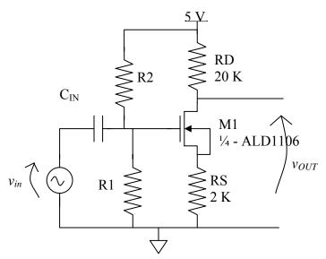
Generally the ALD1106 transistors carry much less current and have lower transconductance than the 2N2222A. The choices of RD and RS reflect that fact – in our 2N2222A example, the equivalent values were 1 K and 100 ohms. When I measured an ALD1106 for lab 2 a couple of years ago, I fitted the following parameters to the data: (This fit was the basis for the recent class handout showing you the meas-
