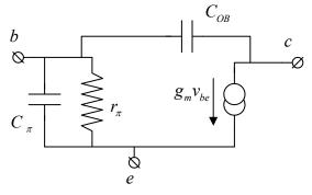
$C_{OB}$  is the capacitance of a reverse biased junction and often has the dependence on voltage of an abrupt-junction. For at least one value of collector-base voltage, it is straightforwardly shown on any datasheet. The transconductance and the dynamic resistance of the base-emitter junction are needed first before one can tease the value of  $C_{\pi}$  out of
