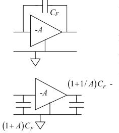
the current in the capacitor is generally greater than it would be if the capacitor were across the input to ground. The theorem points out that this is equivalent to a larger, possibly frequency-dependent capacitor across the input and a marginally bigger one across the output. What often makes this theorem useful is that the low frequency gain is known and that gain is constant enough to use over most of the useful frequency range of the amplifier.
