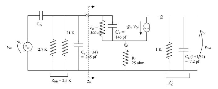
For  $Z_{in}$  we have (neglecting  $C_{IN}$  because it provides only a low-pass cutoff):
