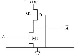
11. The circuit below is a simple gate realized in an unusual way. What Boolean function does it realize? Draw the complete actual transistor version of the circuit. In doing so, assume that both B and its complement are available as inputs. [This type of gate has some advantages in certain circumstances because when embedded in a large system, it is easier to test for manufacturing faults. For a discussion of this issue, see M. Katoozi and M Soma, IEEE JSSC 23 (Oct. 1988) 1241-1248.] VDD
