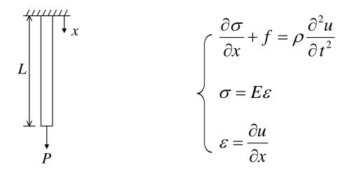
We can consider two simple problems, one with traction BC and one with displacement BC.
