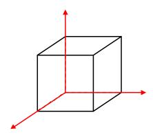
$$\mathbf{C}:\begin{pmatrix} C_{11} & C_{12} & C_{12} & 0 & 0 & 0 \\ & C_{11} & C_{12} & 0 & 0 & 0 \\ & & C_{11} & 0 & 0 & 0 \\ & & & C_{44} & 0 & 0 \\ & & & & C_{44} & 0 \\ & & & & & C_{44} \end{pmatrix} \tag{3 elastic constants}$$
