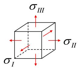
Consider a linear superposition of strain in the principal stress directions
