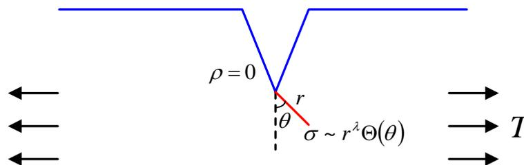
We note that for crack-like flaws,  $\sigma_{\max} \rightarrow \infty$  when  $\rho \rightarrow 0$ , which presents a challenge for failure analysis. Fracture mechanics developed in the mid-20<sup>th</sup> century shows that elasticity solutions for such flaws generally have the form of  $\sigma = Kr^{-\frac{1}{2}}\Theta(\theta)$ .
