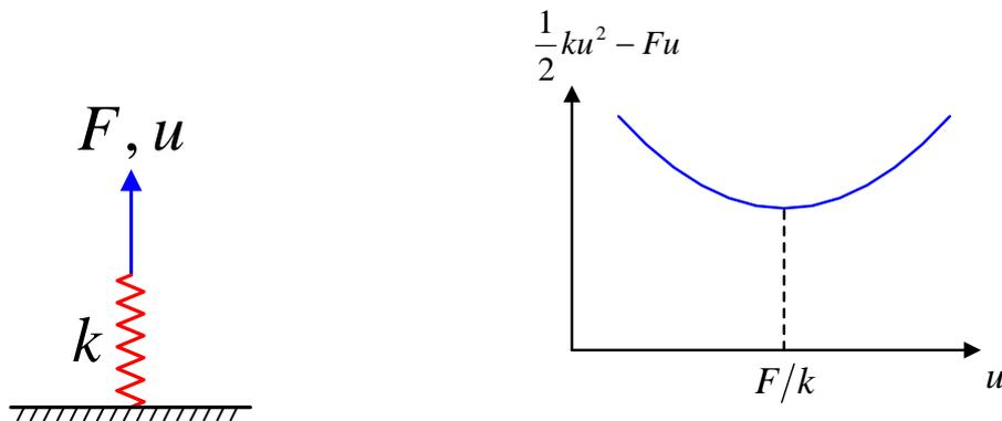
Consider a 1D linear spring under applied force, the potential energy of the system is
