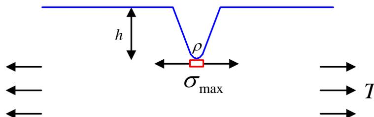
the maximum stress occurs at the crack/notch tip can be expressed as
