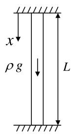
$$K_{ab} = \int_{V} E \frac{\partial N^{a}}{\partial x} \frac{\partial N^{b}}{\partial x} dV = S \int_{0}^{L} E \frac{\partial N^{a}}{\partial x} \frac{\partial N^{b}}{\partial x} dx$$
