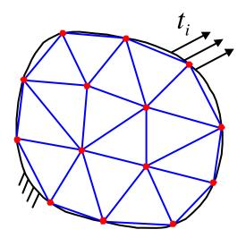
We can represent the displacement by interpolation through its values at a network of nodes (discretization),
