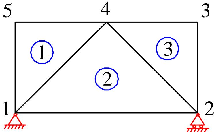
At node 1, the displacements at both directions are fixed; at node 2, the displacement in 2-direction is fixed. The global displacement vector becomes
