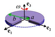
Use the principle of superposition to determine the stress state in a spinning disk with a (traction free) hole with radius *a* at its center.
