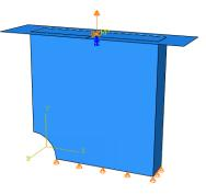
the reference point has U1=U3=0 and a prescribed value for U2 (a load could be applied in the 2 direction as well); and UR2 =0 to remove the rotational mode about the y axis.
