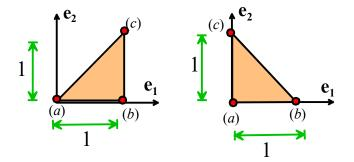
We can use the lengths of the sides of the element and the relation between Lagrange strain and the lengths of material fibers before and after deformation
