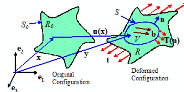
Approximate [small deformation]  $\frac{\partial \bar{\sigma}_{ij}}{\partial x_i} + \rho_0 b_j = \rho_0 \frac{\partial u_j}{\partial t}$  [NLGEOM off]
