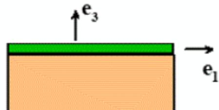
**Example:** A thin film with Young's modulus  $E$ , Poisson's ratio  $\nu$ , yield stress  $Y_0$  and thermal expansion coefficient  $\alpha$  is bonded to a large rigid substrate (with  $\alpha = 0$ ). It is heated by temperature change  $\Delta T$ . Find the value  $\Delta T_y$  that will cause yield.
