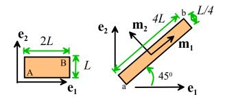
The Cauchy stress in the solid is  $\sigma \mathbf{m}_1 \otimes \mathbf{m}_1$ . Determine:
