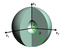
6.1 Assume that the velocity field in the shell is radial  $\mathbf{v} = v(r)\mathbf{e}_r$ . Calculate the velocity gradient and stretch rate.
