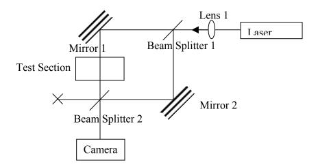
Set up the Mach Zehnder interferometer as shown above and perform the experiments as follows.
