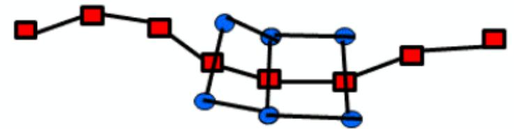
(2) Create a mesh of quadrilateral elements using slaves
