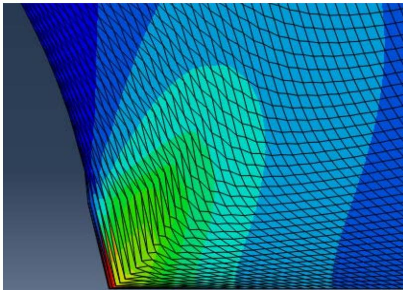
Figure 7: Detail of the deformation of the elements (structured mesh) at the crack tip. The contours show levels of  $\sigma_{22}$ .
