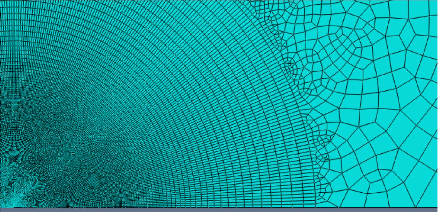
Figure 11: The three partitions of the mesh around the crack tip. From inside out: sweep, sweep, free. The deformation state around the crack tip is similar to that in figure 10. Here, the 1000x Refinement Model is shown.
