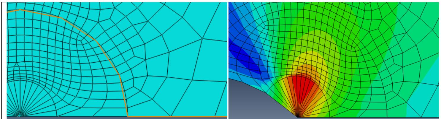
Figure 10: The coarse mesh (Baseline) for sweep-structured-free meshing. *Left*: undeformed, *right*: deformed.
