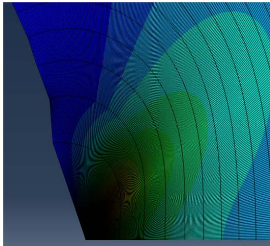
Figure 9: Detail of the deformation of the elements (sweep mesh) at the crack tip. The contours show levels of  $\sigma_{22}$ .
