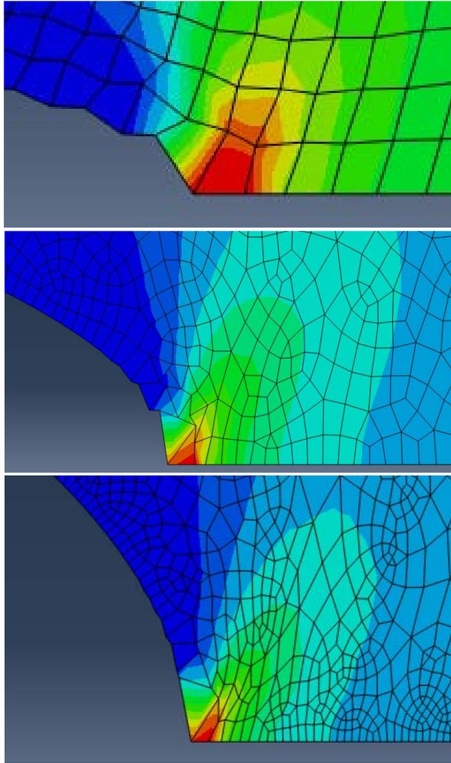
Figure 6: Mesh,  $u_2$ , and  $\sigma_{22}$  around the crack-tip for 2x, 20x, and 100x Refinement (top to bottom).
