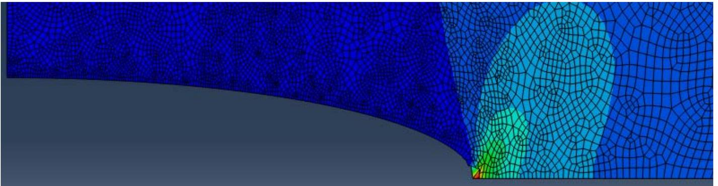
Figure 4: Mesh,  $u_2$ , and  $\sigma_{22}$  around the crack for 20x Refinement
