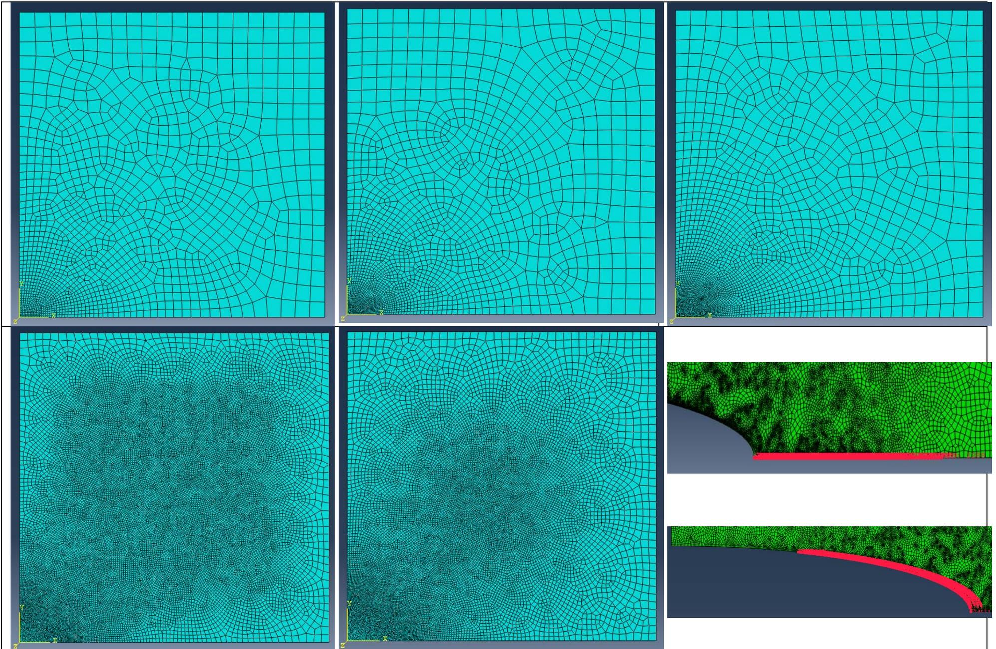
Figure 1: From top-left corner to bottom right: The complete mesh of the body for gradual refinements: Baseline Model, and 2x, 10x, 20x, 100x Refinements (14x Refinement not shown). Here only the edges are partitioned (not the faces) and seeded separately. The mesh type is free.
