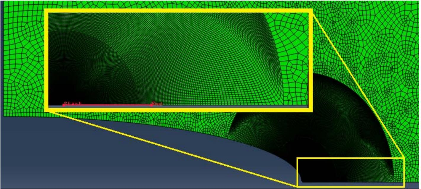
Figure 8: The three partitions around the crack tip. The mesh is increased close to the crack tip (100x). The crack front path for data extraction is also shown. Scale: the total width of the solid is 20, the crack length is 1, and the red path-line is 0.1. Note that the inset is in the undeformed state and the region is approximately mapped for illustration purposes.
