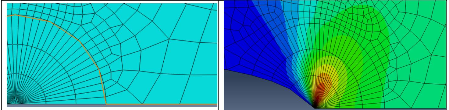
Figure 12: The coarse mesh (Baseline) for sweep-structured-free meshing. *Left*: undeformed, *right*: deformed.
