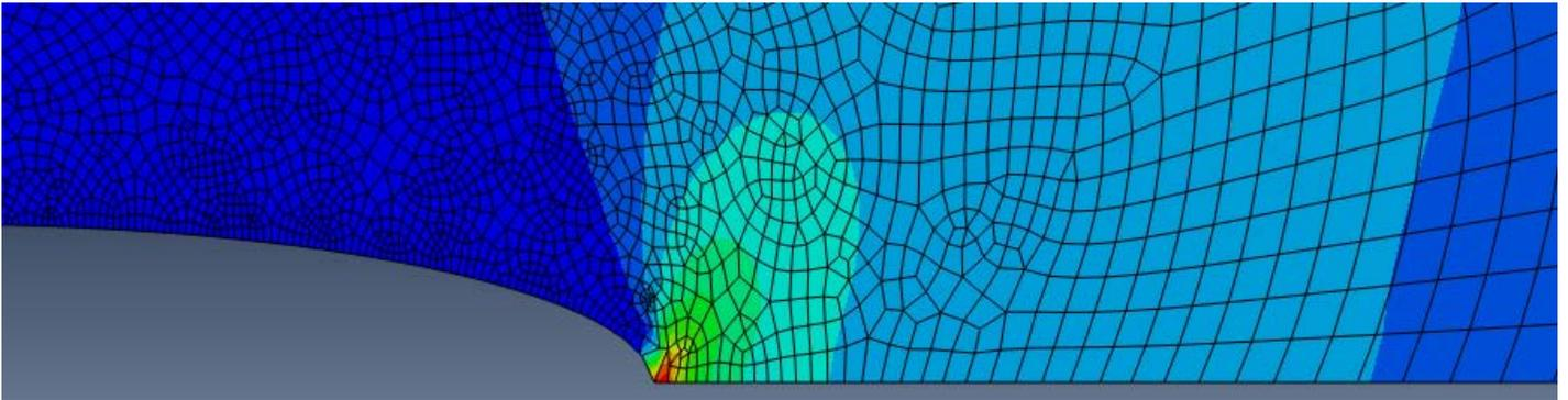
Figure 3: Mesh,  $u_2$ , and  $\sigma_{22}$  around the crack for 10x Refinement
