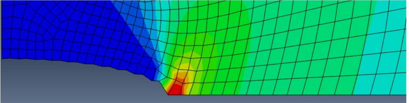
Figure 2: Mesh,  $u_2$ , and  $\sigma_{22}$  around the crack for 2x Refinement
