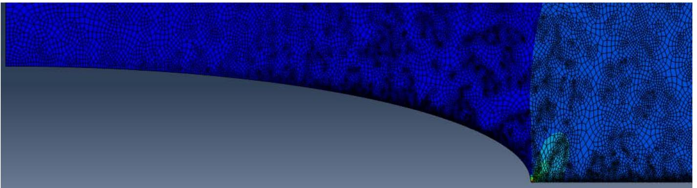
Figure 5: Mesh,  $u_2$ , and  $\sigma_{22}$  around the crack for 100x Refinement
