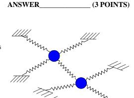
2. How many natural frequencies of vibration are there for the system of masses and springs shown, assuming that the motion is confined to the plane of the page?
