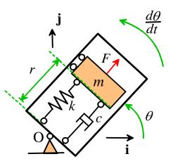
The goal of this problem is to derive an equation that relates the resonant frequency  $\omega^*$  to  $d\theta/dt$ .
