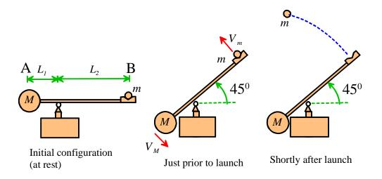
**11.** (15 pts) A proposed design for a catapult that launches a projectile with mass m is shown in the figure. The mass of the arm AB can be neglected, and the masses m and M can be idealized as particles.
