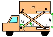
14.1 Write down the height h of the mass m in terms of  $\theta$ . Hence, determine a formula for the vertical speed dh/dt of the payload in terms of  $d\theta/dt$  and any other relevant variables.
