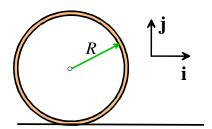
13.1 Draw the free body diagram for the ring just after it comes into contact with the surface.
