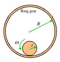
The points on the two bodies where they touch must have the same velocities. So  $\omega r = \omega_r R \Rightarrow \omega_r = \omega r / R$  and since this is positive the rotation direction is counterclockwise
