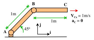
12.1 Determine formulas for the velocity vectors  $\mathbf{v}_B, \mathbf{v}_C$  of points B and C, in terms of  $\omega_{AB}, \omega_{BC}$ . (You do not need to solve for  $\omega_{AB}, \omega_{BC}$  until 12.3).
