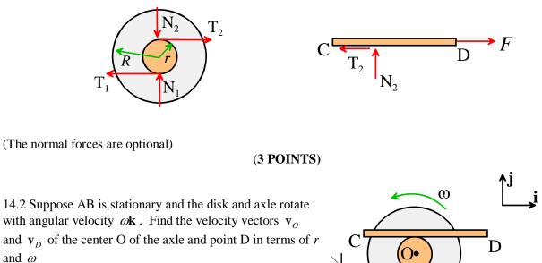
The wheel rolls without slip on the member AB. The center therefore has velocity  $\mathbf{v}_{o} = -\omega r \mathbf{i}$ . There is no slip at the contact between the axle and CD. D therefore moves with the same velocity as the axle at the contact point – this is  $\mathbf{v}_{D} = -2\omega r \mathbf{i}$
