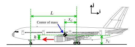
4.1 Draw the forces acting on the aircraft on the figure provided below (you can represent the forces acting on the rear wheels as a single statically equivalent force).
