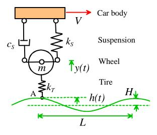
The wheel vibrates vertically with a displacement from its static equilibrium position y(t). Vertical motion of the car body can be neglected.
