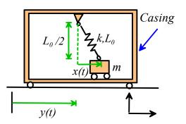
3.1Draw a free body diagram showing the forces acting on the mass. Gravity may be neglected
