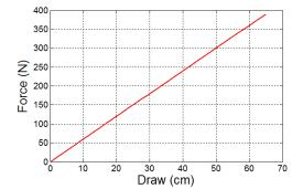
The dynamic efficiency is the ratio of the KE of the arrow to the energy stored in the
