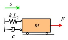
At time t=0 the system is at rest, and F=0. At time t=1s a constant force of F=100N is applied to the mass. The figure below shows the variation of s with time for 0 < t < 5s.
