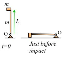
22.1 Find the total mass moment of inertia of the system (the rod together with the hammer-head) about O
