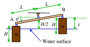
The goal of this problem is to analyze oscillation of the device in still water (no waves). No torque or friction acts at the pivot. Neglect the mass of AB and viscous drag of the water.
