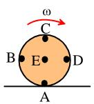
The wheel is instantaneously rotating about A so the point furthest from A has the greatest speed.
