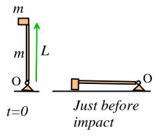
22.1 Find the total mass moment of inertia of the system (the rod together with the hammer-head) about O
