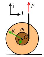
22.4 Use 22.2 and 22.3 to find formulas for (a) the angular acceleration and (b) the linear acceleration of the spool in terms of P, and other relevant variables.
