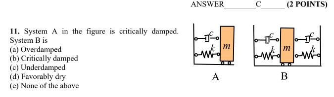
The damping factor for A is  $\zeta = c/2\sqrt{km} = 1$ . Since the springs and dashpots are in parallel the damping factor for B is  $\zeta = 2c/2\sqrt{2km} = \sqrt{2} > 1$  so the system is overdamped.
