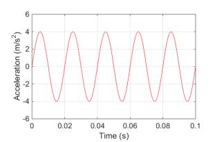
The amplitude of the acceleration is 4 m/s<sup>2</sup> and the period is 0.02s. The angular frequency is therefore  $\omega = 2\pi / 0.02 = 100\pi$ . The displacement amplitude follows as  $X_0 = A_0 / \omega^2 = 4 / (10000\pi^2) \approx 41 \mu \text{ m}$
