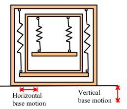
There are two moving masses in the system, each of which is a rigid body that can translate freely in both horizontal and vertical directions, and can rotate about the **k** axis. This is 2x3=6 DOF. There are no rigid body modes so 6 vibration modes.
