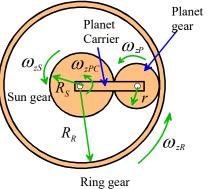
The general formula relating angular velocities in a planetary Rigear system is  $(\omega_{zR} - \omega_{zPC})/(\omega_{zS} - \omega_{zPC}) = -(N_S / N_R)$ Substituting numbers given  $-\omega_{zPC}/(3\omega_{zPC} - \omega_{zPC}) = -20 / N_R \Rightarrow N_R = 40$ . Finally  $2N_P = N_R - N_S \Rightarrow N_P = 10$
