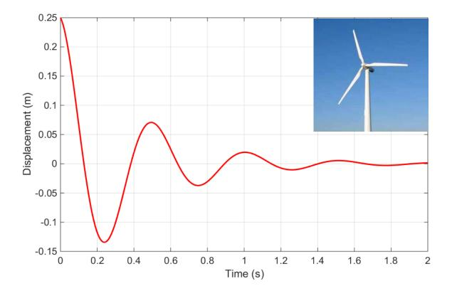
**21** An unbalanced wind-turbine is idealized as a rotor-excited springmass system as shown in the figure. The mass *m* represents the tower, and  $m_0$  represents the combined mass of the three rotor blades. The spring and damper represent the stiffness and energy dissipation in the tower. The rotor is 'unbalanced' because its center of mass is a small distance  $Y_0$  away from the axle. The total mass  $(m + m_0)$  of the system is 25000kg.
