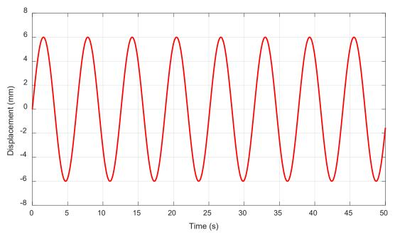
21.2 The figure shows the measured displacement of the system during operation. The blades have a radius of 40m, and the total mass of the system  $(m + m_0)$  is 25000kg. Assuming that the rotor can be balanced by adding mass to the tip of one blade, estimate the mass that must be added to balance the rotor.
