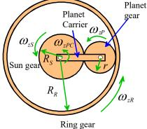
The general formula relating angular velocities in a planetary Ring gear gear system is  $(\omega_{zR} - \omega_{zPC})/(\omega_{zS} - \omega_{zPC}) = -(N_S / N_R)$ Substituting numbers given  $(3\omega_{zPC} - 2\omega_{zPC})/(0 - 2\omega_{zPC}) = -20 / N_R \Rightarrow N_R = 40$ . Finally  $2N_P = N_R - N_S \Rightarrow N_P = 10$
