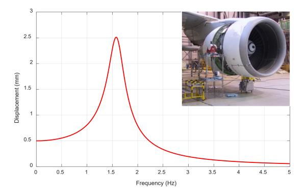
**21** As part of the airworthiness certification process, the rotating parts of a jet engine are prevented from turning, and the engine is subjected to an external horizontal harmonic force  $F(t) = F_0 \sin \omega t$  with amplitude  $F_0 = 250$ N. The amplitude  $X_0$  of the steady-state horizontal vibration  $x(t) = X_0 \sin(\omega t + \phi)$  of the engine is measured.
