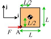
The mass moment of inertia of the plate is  $I_{Gzz} = mL^2/12$  (given). Taking moments about the center of the plate, the equations of motion are  $F\mathbf{i} = m\mathbf{a}_G$   $(FL/2)\mathbf{k} = I_{Gzz}\alpha\mathbf{k} \Rightarrow \alpha = 6F/(mL)$ . The acceleration of point A is  $\mathbf{a}_A = \mathbf{a}_G + \alpha\mathbf{k} \times (-(L/2)\mathbf{i} - (L/2)\mathbf{j}) = (F/m)\mathbf{i} + (3F/m)\mathbf{i} - 3(F/m)\mathbf{j}$
