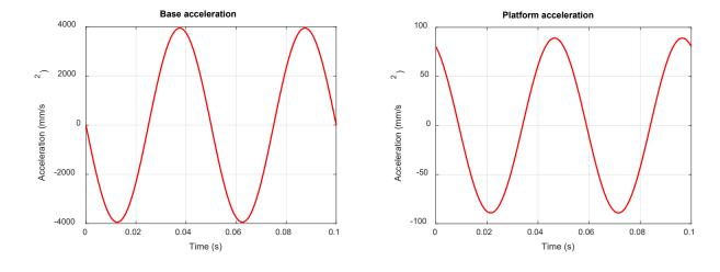
**21** The figure shows readings from accelerometers attached to the base and platform of a vibration isolation table.
