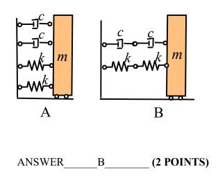
The springs/dashpots in A are in parallel; in B they are in series. Therefore  $\omega_{nA} = \sqrt{2k/m} \quad \zeta_A = 2c/(2\sqrt{2km})$  and  $\omega_{nB} = \sqrt{k/2m} \quad \zeta_B = c/4\sqrt{km/2}$  giving (b)
