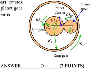
Use method from class – consider motion of system in a reference frame rotating with planet carrier  $(\omega_{zP} - \omega_{zPC}) / (\omega_{zS} - \omega_{zPC}) = -R_S / r \Rightarrow \omega_{zPC} (1 + R_S / r) = \omega_{zS} R_S / r$  and so (d)
