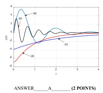
Rearrange the equation in standard form  $\frac{1}{4^2}\frac{d^2y}{dt^2} + \frac{2 \times 0.25}{4}\frac{dy}{dt} + y = 0$  showing that  $\omega_n = 4$  and  $\zeta = 0.25$ . This is an underdamped solution with period approximately  $2\pi/4$ ; i.e. (a)
