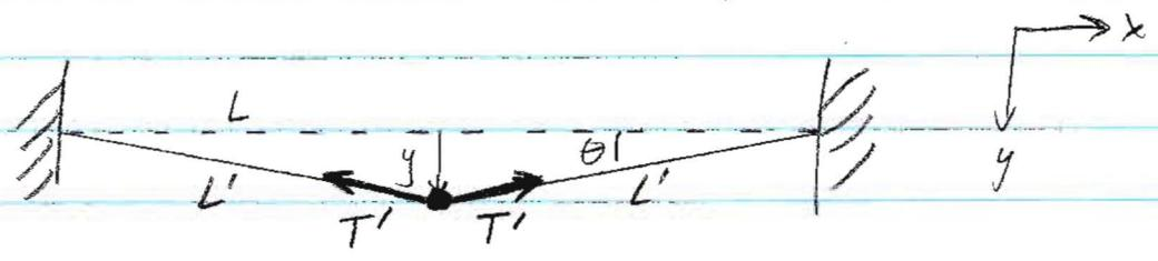
Tension  $T'$  is unknown at the moment. When  $y=0$ , tension is  $T$ . For  $y \neq 0$ , the tension  $T'$  will change due to the change in length of the wire. However, that change in length is quite small, so that  $T' = T$  is accurate for  $y/L \ll 1$ .
