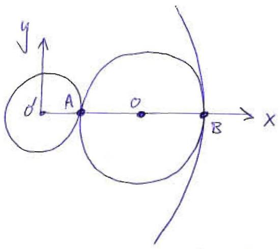
Identify points A, B at contacts of sun, planet gears and planet, ring gears, respectively. Let O be at center of planet gear.
