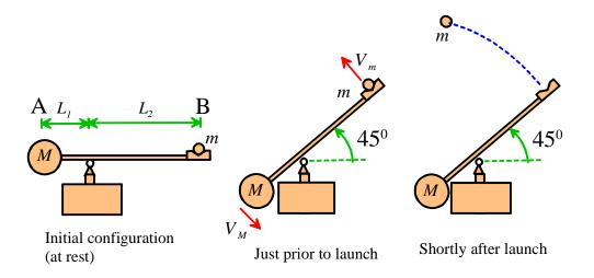
4. A proposed design for a catapult that launches a projectile with mass *m* is shown in the figure. The mass of the arm AB can be neglected, and the masses *m* and *M* can be idealized as particles.
