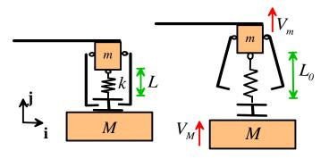
equal and opposite impulses on the specimen and the test mass m.
