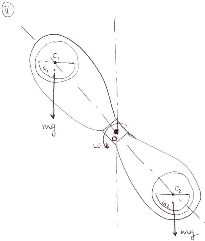
Consider the wheel at some point during its operation as shown above. The center of mass of each load is directly below its center of rotation, i.e.  $G_1$  is always 1m below  $C_1$  and  $G_2$  is always 1m below  $C_2$ . So the velocity of  $G_1$  is the same as that of  $C_1$ ; the velocity of  $G_2$  is the same as that of  $C_2$ .
