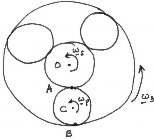
$$\text{Given : } \underline{\omega}_s = -\omega_1 \underline{k}$$
