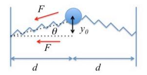
4.5 What is the natural frequency of the small oscillations along the *y* axis? **solution** [1 point]
