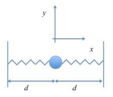
4.1 The mass is given a displacement of  $x_0$  to the right. Give equations for  $F_1$  and  $F_2$ , the forces exerted by the two springs. Use the sign convention that a positive force acts toward +x.
